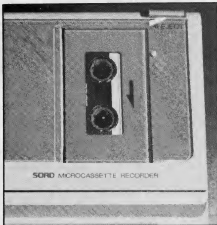
Microcassette recorder operates at 2000 baud; a C-30 cassette can store 128K of data.
